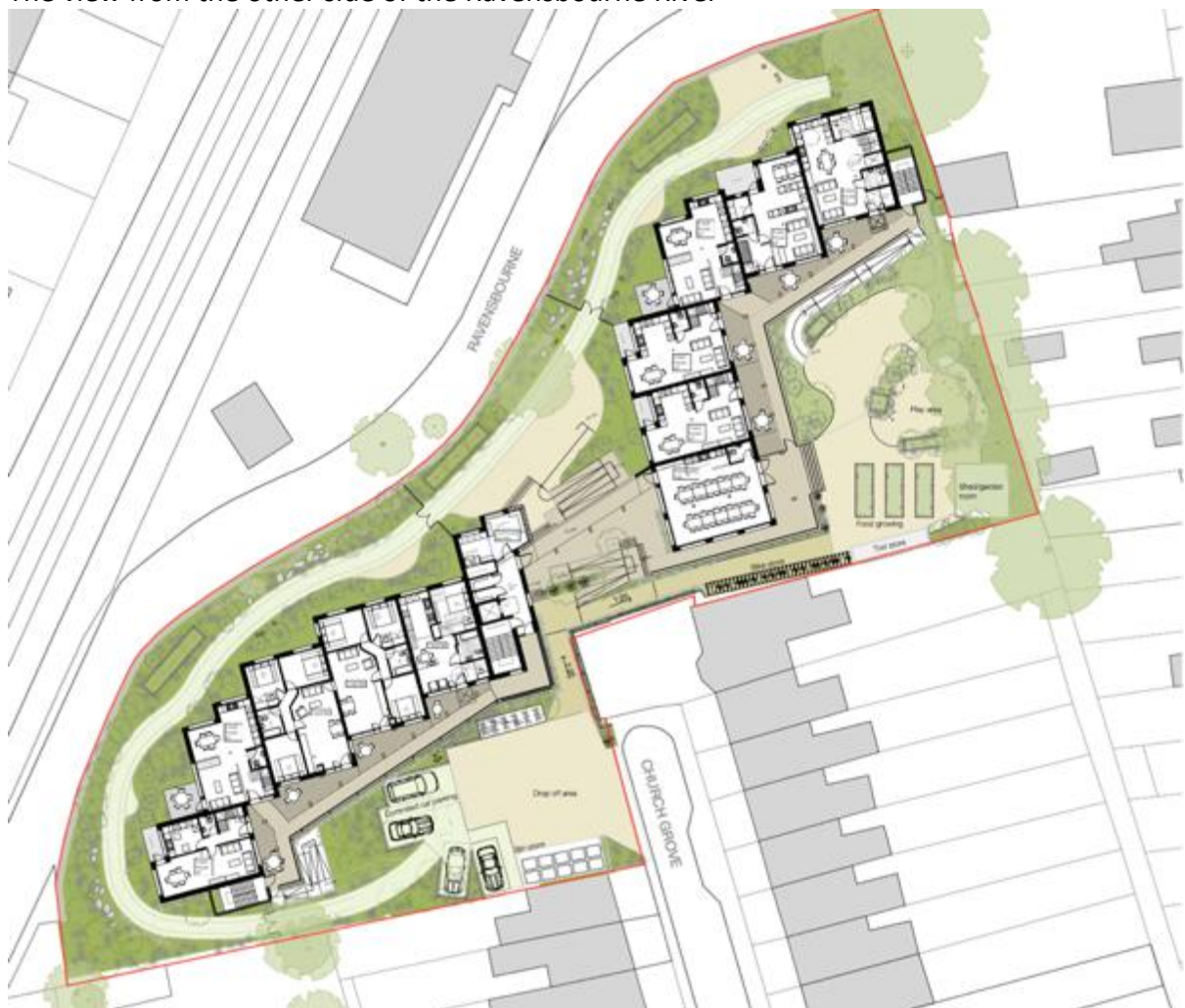
Ground floor plan showing the two main blocks, the new common space/community facility and the nature trail alongside the river
